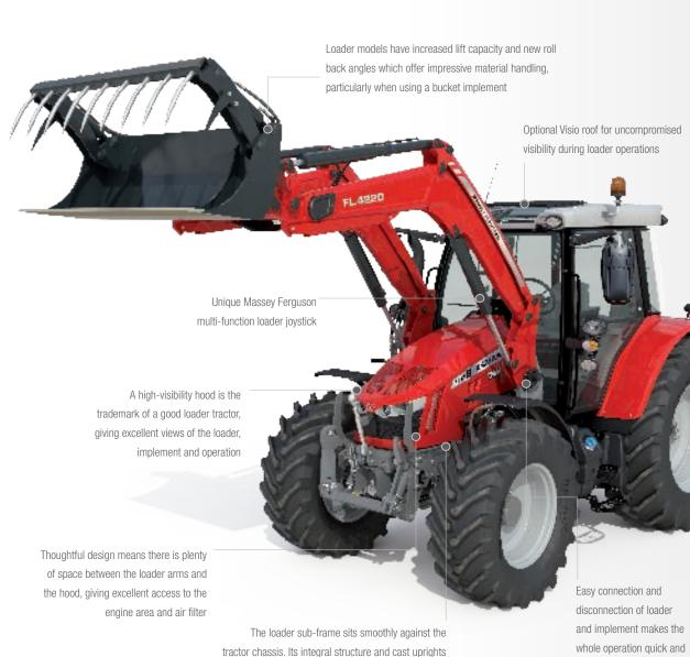
have been carefully designed by our engineers who understand how a tractor and loader need to perform
