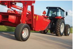
**THE HIGH-CLEARANCE MAINFRAME** provides an exceptional header lift height of 20 inches for better clearance over headland windrows. The added height also allows the header to be easily carried over obstacles, ditches and waterways.
