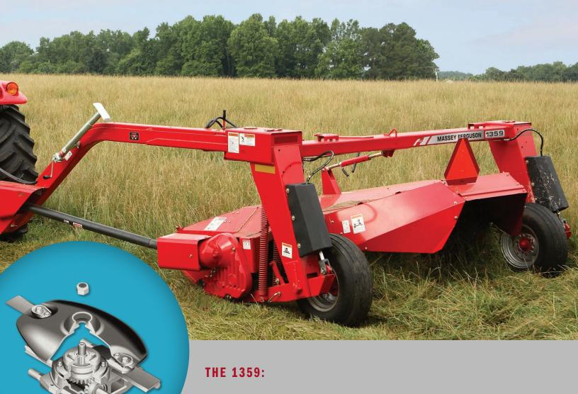
Standard knives feature a 12-degree pitch. For tough conditions like down crop, 18-degree knives are also available for more lift and a cleaner cut.
